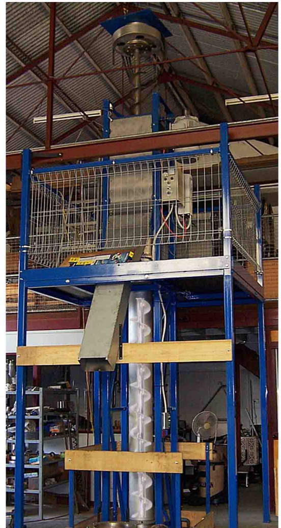
10" (250mm) Olds Elevator test facility
