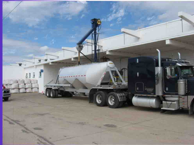
An 8" (200mm) Olds Elevator installed at a Chemical company filling tankers at 35T/Hr
