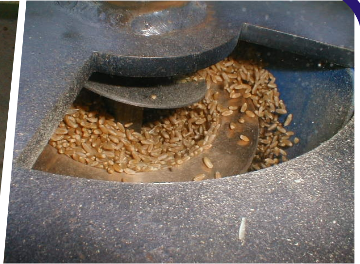
View in top - product spilling over and down
